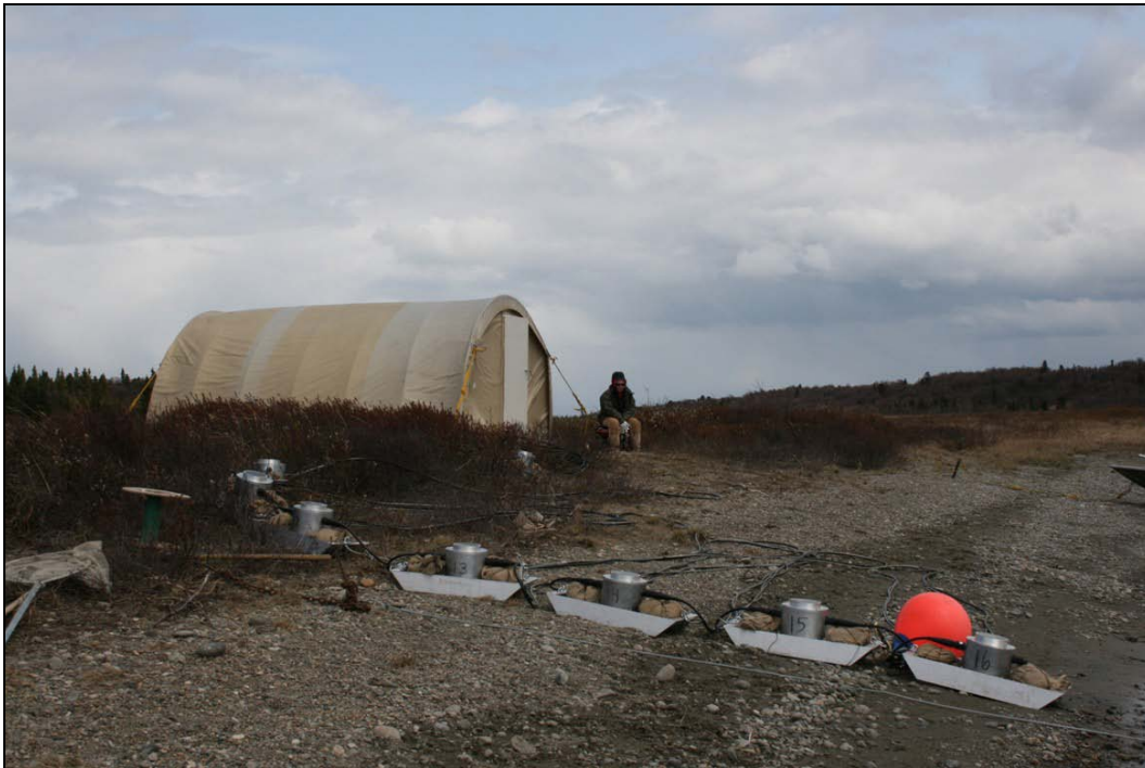
Photo 2. Sonar array of 8 pods staged at Site 1 on the river's west bank with the WeatherPORT tent in the background, 2008.
