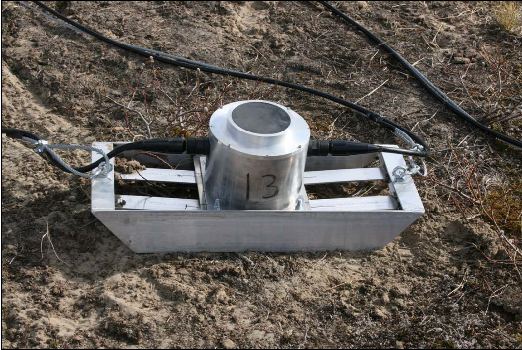
Photo 1. Up looking transducer mounted on sled with attached power and tow cables used in the Kvichak River, 2008.
